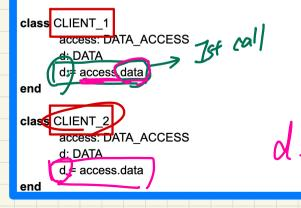
Since DATA\_ACCESS is an expanded class, both `access` objects in these clients would be different instances of DATA\_ACCESS.
